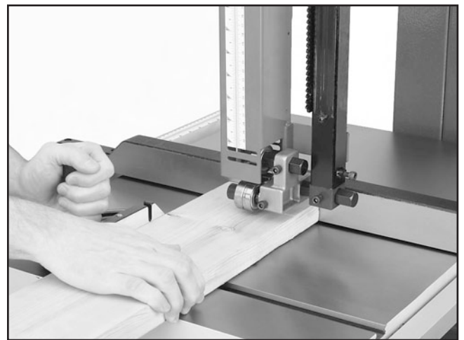
Figure 44. Crosscutting with miter gauge.
